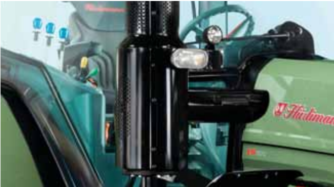
Modernste SCR (Selective Catalyst Reduction) Abgastechnologie.
